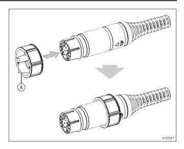
2. Slide the split-ring over the end of the connector, then push it towards the cable-end of the connector.
