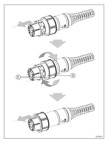
The locking collar slides easily towards the plug-end of the connector, before butting up against the split-ring moulding.
