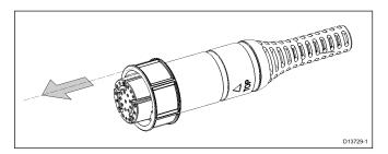
As you pull the locking collar, it clicks into place over the split-ring. The locking collar stays in position on the connector, but rotates freely.
