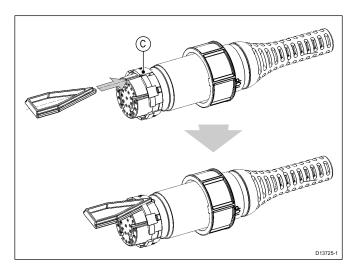
The tool widens the gap in the split ring, enabling the split ring to be pushed further back onto the connector in the following step.
