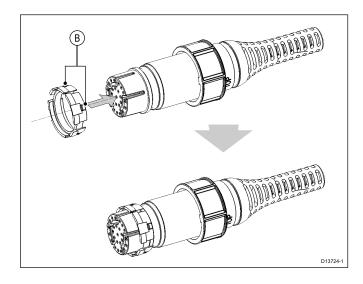
The split-ring slides easily for approximately 1 cm onto the connector, before butting up against the connector moulding.
