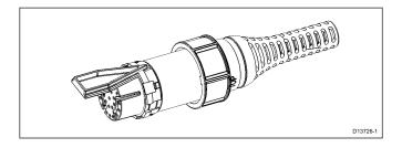
You can now remove the tool. The split-ring stays in position on the connector, but rotates freely.
